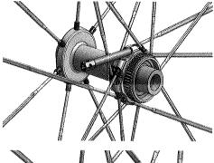
3. Insert the enclosed pin into the tool and unscrew the defective spoke carefully piece by piece.
