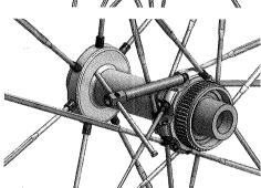
To fit in a new spoke, please clean the thread in the hub, apply Loctite 243 to the spoke thread and turn the spoke into the hub.
